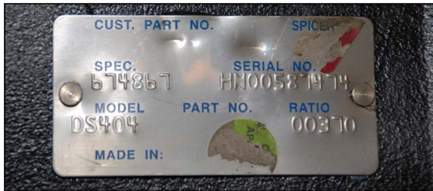
Figure 2 – Sample Spicer Transmission Identification Tag
