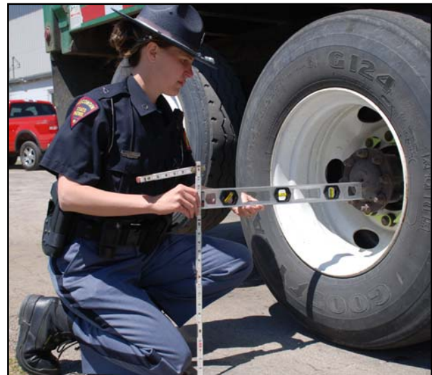
Figure 3 – Measuring Rolling Radius
