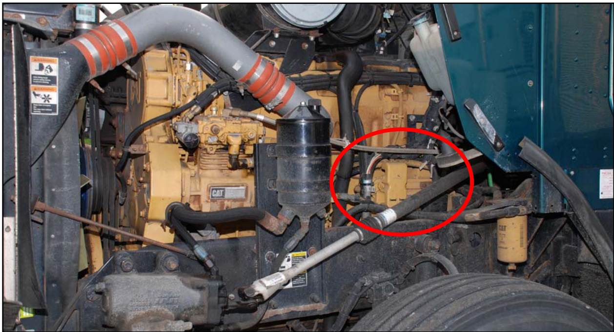
Figure 6 – Sample Caterpillar ECM Location
