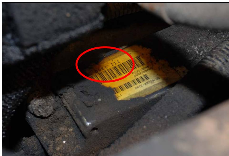
Figure 15 – Sample DDEC III Identification
