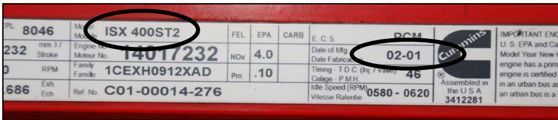
Figure 8 – 2001 Cummins ISX Identification Tag
