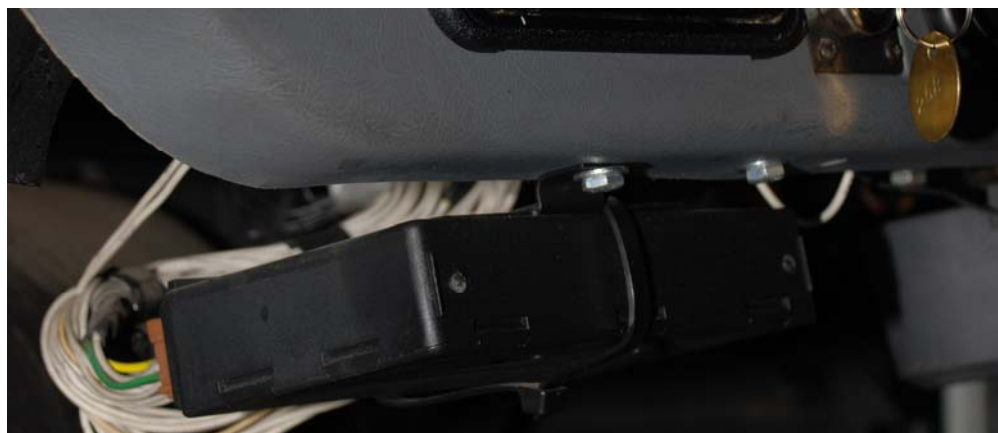
Figure 19 – Sample Mercedes-Benz Vehicle Control Unit (VCU)
