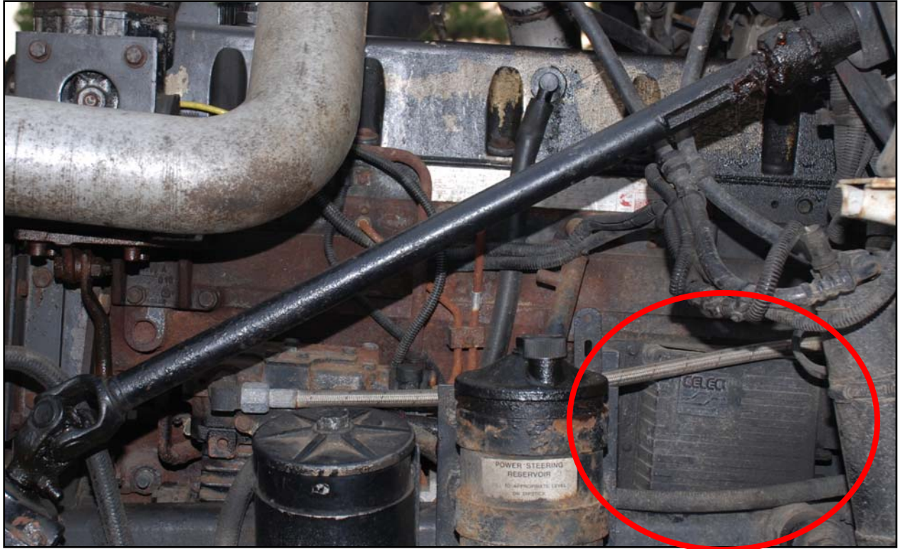
Figure 10 – Celect ECM on 1994 Cummins M11 Engine
