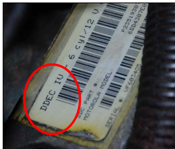
Figure 12 – Detroit Diesel DDEC III and IV Location and Identification Label
